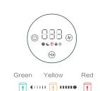
After replacing the new filter element, long press @ and ① for 2 seconds, the filter replacement is completed
